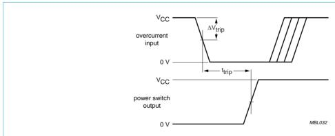
Overcurrent input: OCn; power switch output: PSWn.
